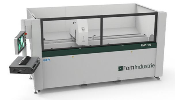
Air-cooled 3kW ISO 30 spindle motor Adjustable motor speed from 1,000 - 15,000 rpm Standard tool magazine has six locations Four cast aluminium pneumatic vices with dual working pressure (high and low) Manual longitudinal postioning Vertical and transversal adjustments do not require tools Two manual stops (left & right side) Control console - Windows 10, USB ports Cloud-based software for monitoring and increasing productivity/efficiency Turnkey system
