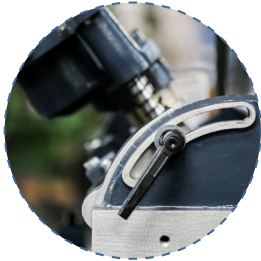
Top motor can be angled for concealed drainage on PVCu profiles
