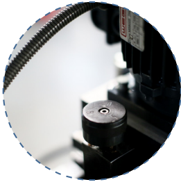
Stylus assembly with 5, 8 & 10mm pins for 1:1 ratio routing
