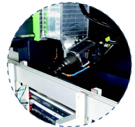
12-axis CNC Controller with RTCP function
